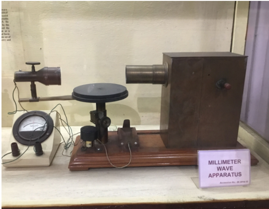
Figure 1a: Millimeter-wave apparatus manufactured by J. C. Bose. Photographed by the author at the Bose Museum, Kolkata.
