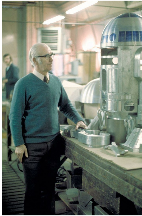
Figure 2. A worker at Peteric Engineering (likely Jack Swinbank) inspects an Artoo unit. The photograph details the droid's thin aluminium sheets and hand-punched details. Photo: provenance unknown, ca. 1976.
